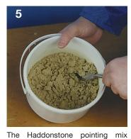
(shown) is ready to use when it has the consistency of damp sand. The TecStone/TecLite pointing mix is ready to use when the consistency of putty. \*See note below.
