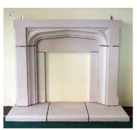
Attach mantel to wall using 100 x 25mm (4" x 1") mild steel straps and pin and bed mantel to legs using 6mm Ø ( $\frac{1}{4}$ ") 100mm (4") long mild steel dowels on a 1:1:6 cement/lime/sand mortar. Repeat this process for the mantel shelf.
