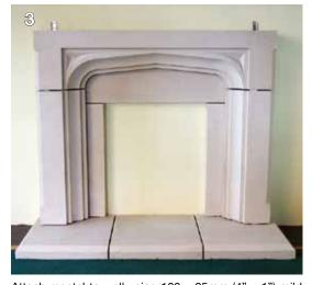
Attach mantel to wall using 100 x 25mm (4" x 1") mild steel straps and pin and bed mantel to legs using 6mm Ø ( $\frac{1}{4}$ ") 100mm (4") long mild steel dowels on a 1:1:6 cement/lime/sand mortar. Repeat this process for the mantel shelf.
