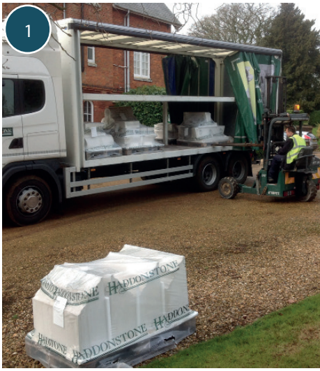
1 Haddonstone delivery on shrink-wrapped pallets incorporating pallet manifests to help identification.
