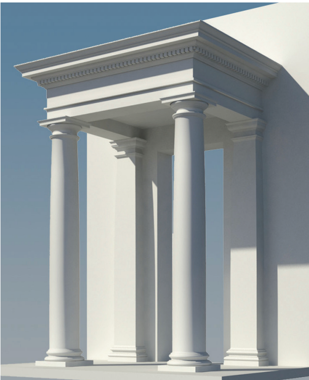
GIBBS III - Doric porch with Dentil Cornice, Architrave and Stepped Frieze
